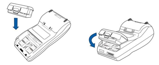
Figure 17 **Installing the Smart Battery**
